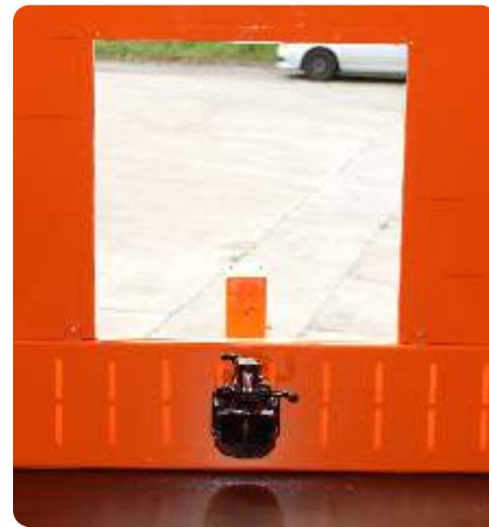
Front wall made of steel sheet with slotted holes for the mounting of couplings in different positions, installation of a Rockinger coupling with a possible remote release on the bulkhead and window to reach through (optional equipment)
