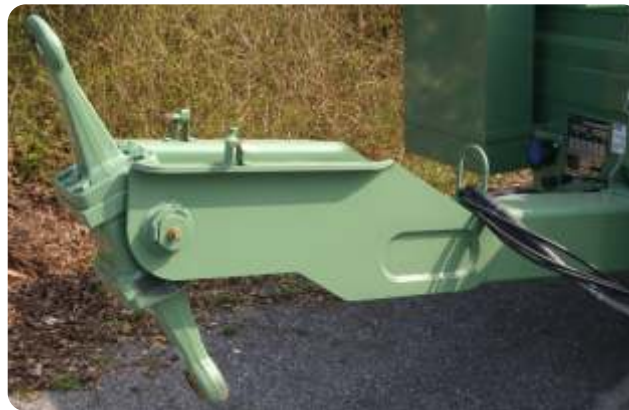
Swivel head with optionally 40mm and 50mm draweye
