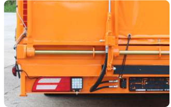
Full LED lighting 24V, additional LED backing lights, ramps widened to 80cm, can be fully pushed together, with gas spring absorbers
