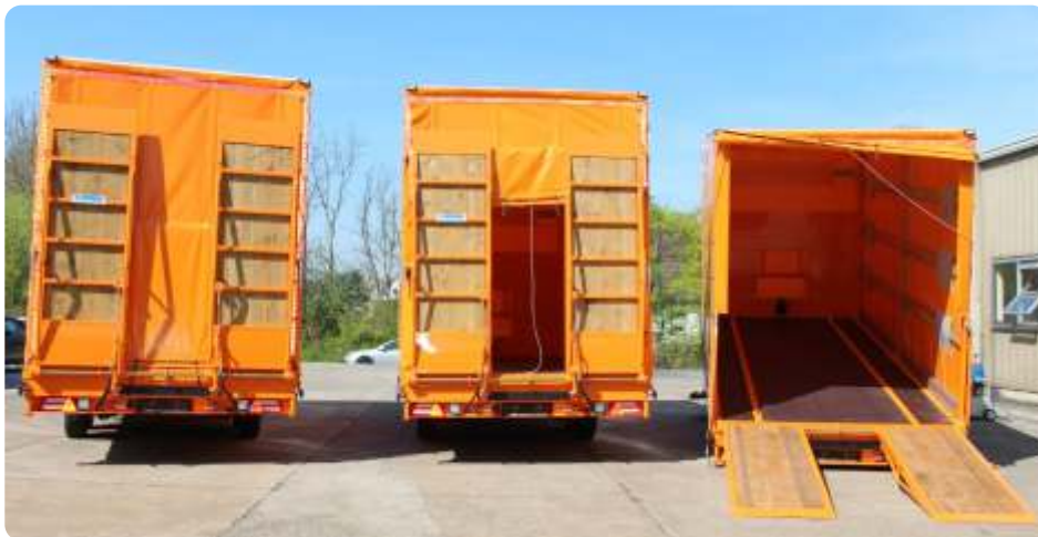
Rear and interior view: Rear roller blind, flashing lights on the body, additional LED reversing light, full LED lighting, widened ramps to 80cm - fully collapsible (partly additional equipment)
