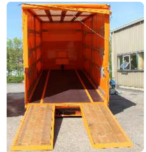
Front wall made of steel sheet with slotted holes for the mounting of couplings in different positions, installation of a Rockinger coupling with a possible remote release on the bulkhead and window to reach through (optional equipment)
