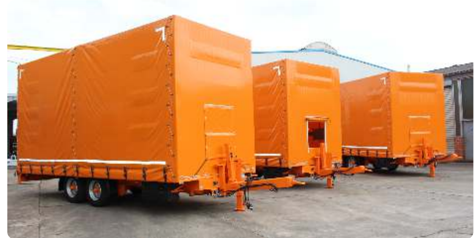
Window for reaching through for releasing the coupling from the front, closable by roller blind, with ascent aid on the front side, height adjustable drawbar (partly additional equipment)
