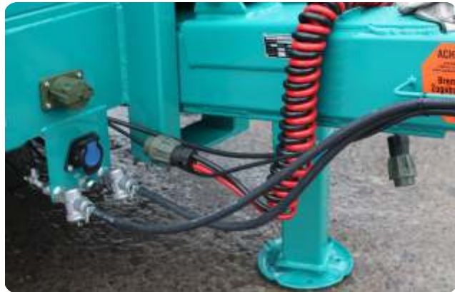
Spiral cable with NATO plug, supply to the towing vehicle
