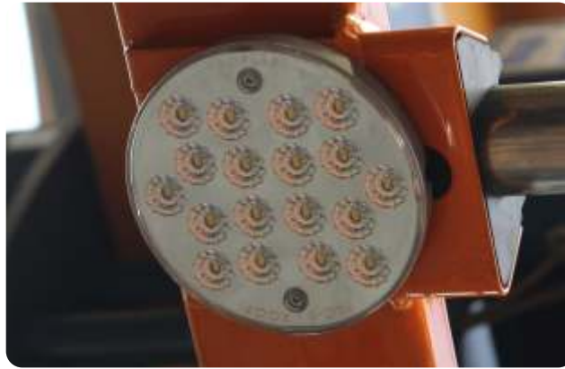
LED interior lighting at the roof, switchable
