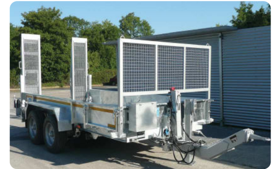
Tool box at the front wall, pluggable front wall elevation, side flap
