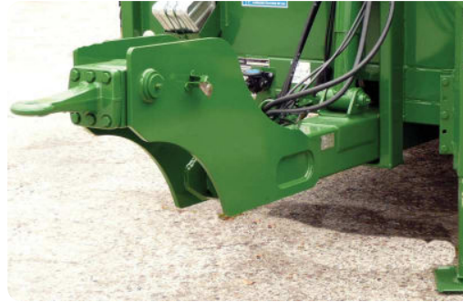
Swinging towing eye - 40 to 50mm towing ring (no COC possible)
