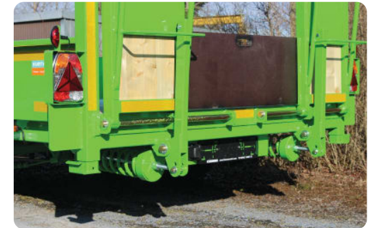
Spring lifting supports for ramps instead of gas pressure absorbers
