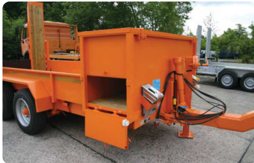
Double storage box with side flaps and top lid for the loading from the top
