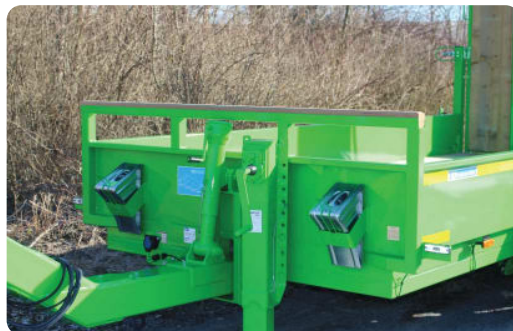
Support frame with hardwood on front wall for excavator shovel
