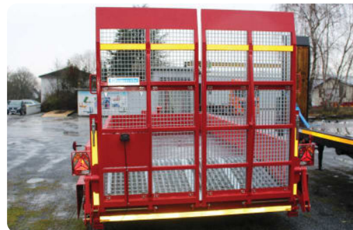
Closed loading ramp, with side protection grids at the slope
