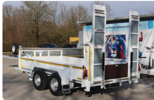
Grids in the ramps - with additional gas pressure absorbers
